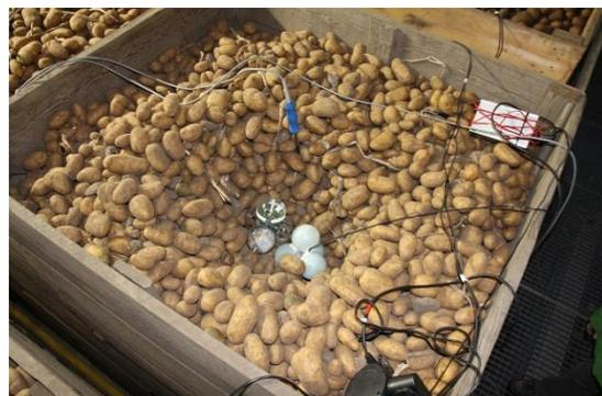
Fig 2. The ASL sensor placed in potatoes
